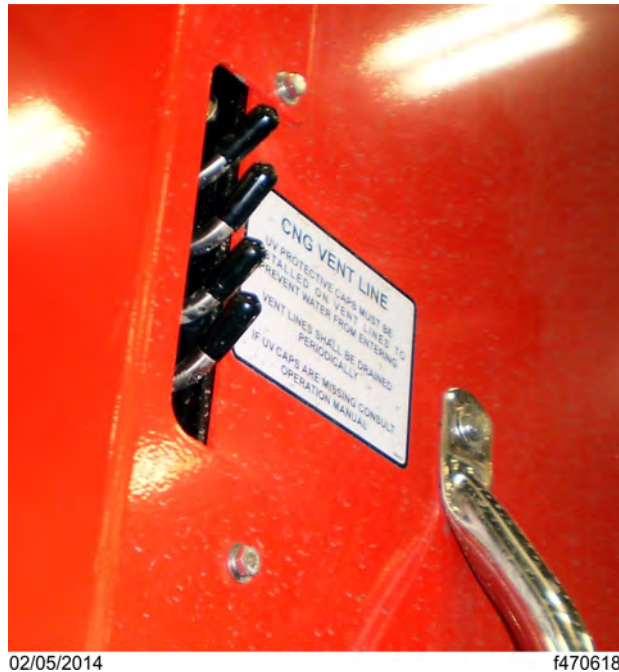
Fig 264, CNG Vent Line Caps
