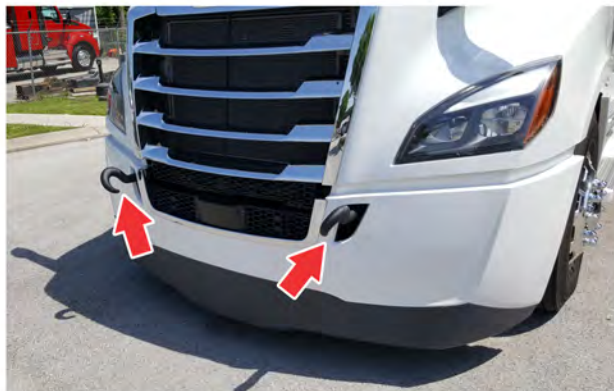
Fig 288, Tow Hooks Installed, Facing Down
